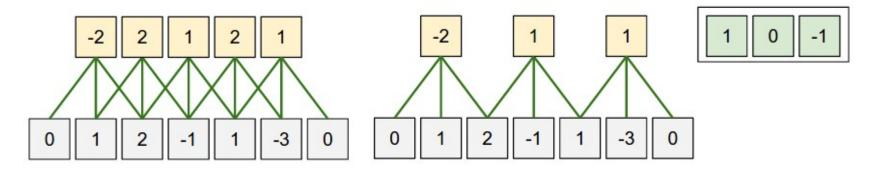
The green sequence [1, 0, -1] is the filter. The signal g is in gray, and the outputs of the convolution
