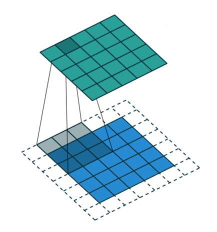
In this example, f is a 3x3 array (gray area). g is a 5x5 array (blue area). The result of the convolution is the top green area.
